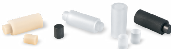
Figure 1. Containers for dilatometer measurements, made of alumina, fused silica, sapphire and graphite
