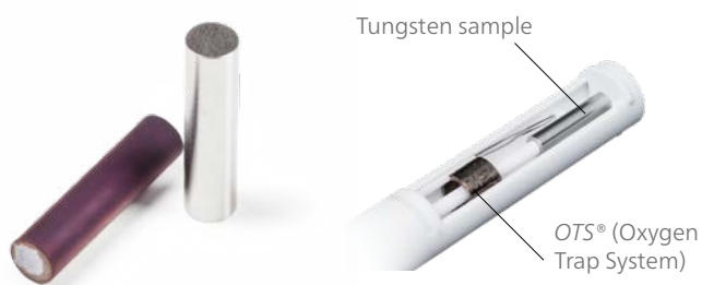
Left: Two tungsten samples after a measurement up to 1640°C. The sample on the left is corroded due to the oxygen-containing test atmosphere; the sample on the right still shines due to a measurement in an oxygen-free test atmosphere.
