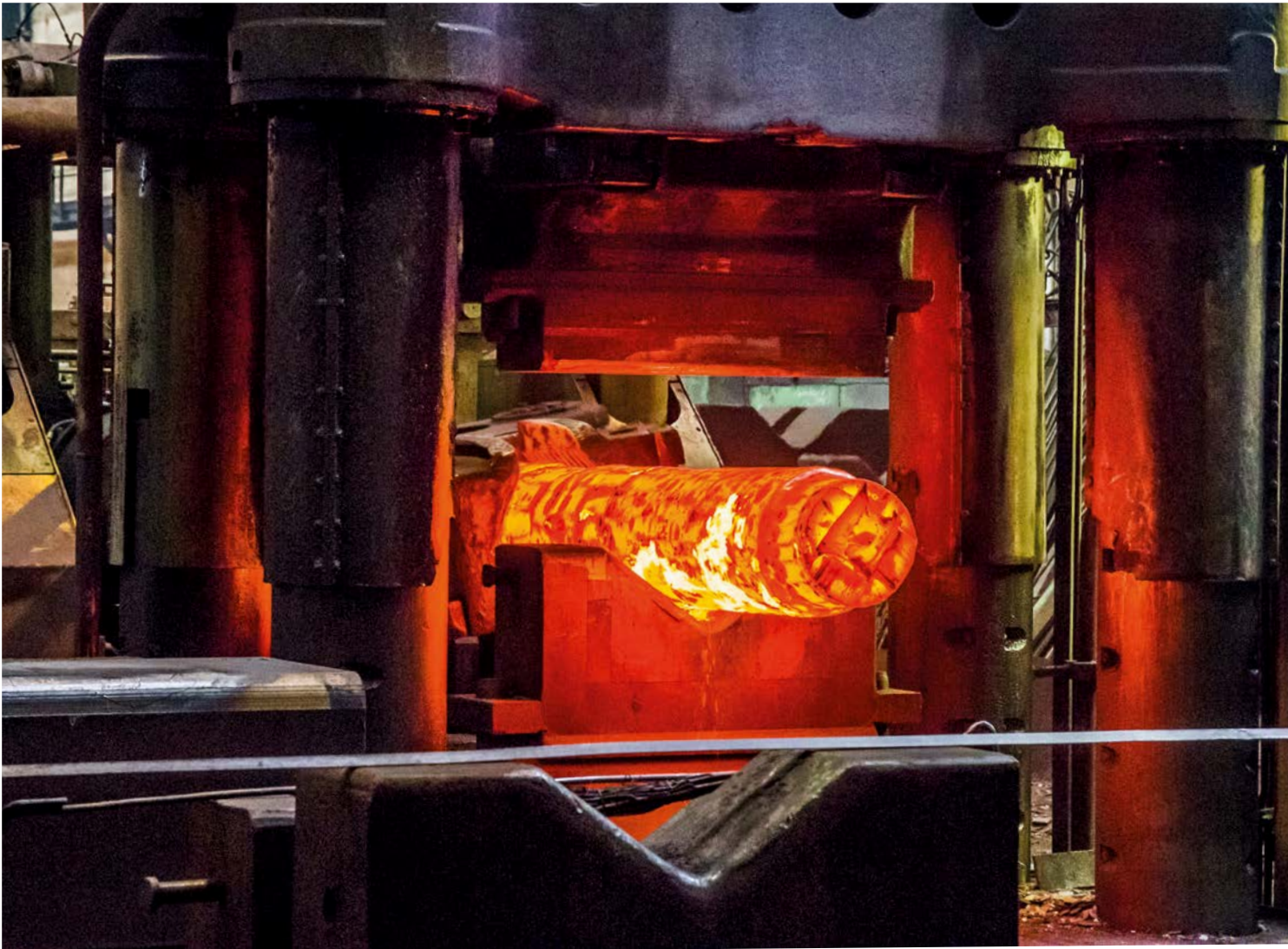
Steel ingot in a hydraulic forging processes
