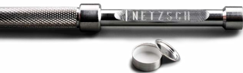
Figure 2. The crucible combination of PtRh/ \text{Al}_2\text{O}_3 can be used for samples which may react with Pt up to 1700^\circ\text{C} . MgO and \text{Y}_2\text{O}_3 liners are also available.
