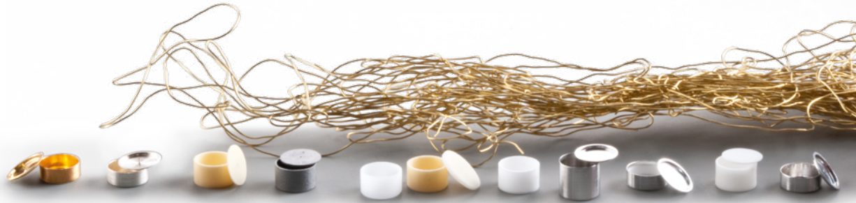
Crucible variety made of Au, Ag, Pt, Al 2 O 3 , BN for NETZSCH STA systems
